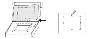
3. Secure the operator terminal in position, using all the fastening holes and the provided brackets and screws:
